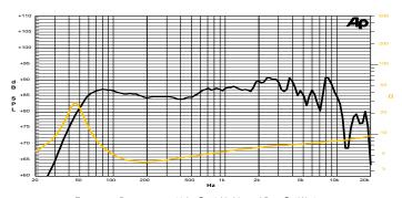
Frequency Response on 18 Lt @ 50 Hz Vented Box @ 1W, 1m Free Air Impedance
